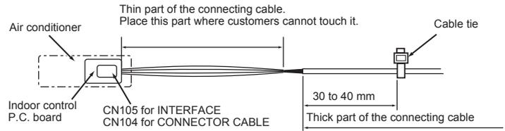
The connector CN104 does not send a signal to a connected external device, but receives a signal from it. An external heater, for example, cannot be connected to CN104 as sending a signal to the external heater is required to turn it on or off.
