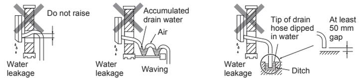
Do not put the drain pipe directly in a drainage ditch where Ammonia or Sulphuric gas may be generated. The evaporated corrosive gas may return to the indoor side through drain pipe and this may cause an unpleasant odor and corrosion on Heat exchanger may occur.
