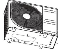
Do not block the drain holes when installing the outdoor unit.
